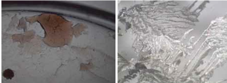
Figure 17: examples of solidified oil and dendritic solidification
