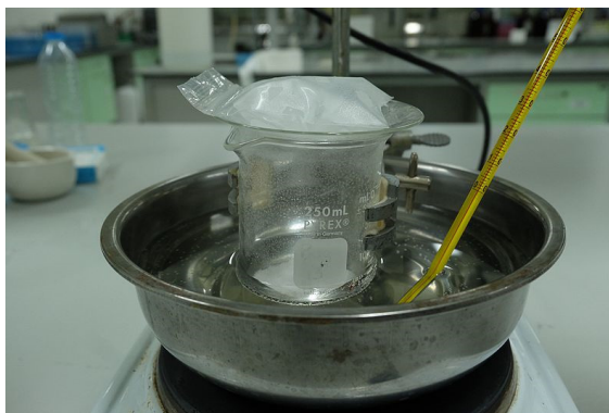
Figure 6: Cold finger and an example of setup: a watch glass used as cold surface
